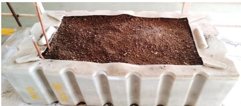
Figure.2 Actual working EHE system with buried pipe in the soil
