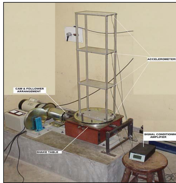
Figure 3.5: Test model of a three-story house on a shake table
