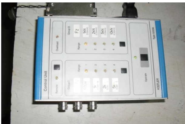
Fig.3. Photograph of KISTLER dynamometer (a) Control box and (b) GFRP composite mounted on dynamometer
