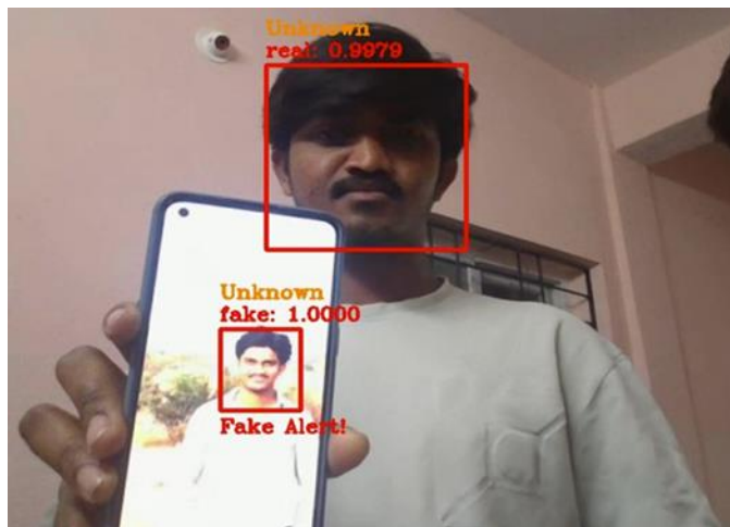
Fig. 6. Real-time identification of both live and spoof faces in one evaluation scenario
