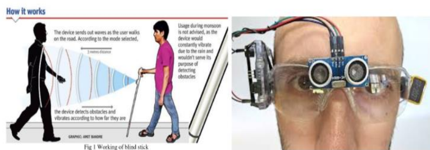
Fig 1. Ultrasonic sensor-based obstacle detection system for visually impaired users.
