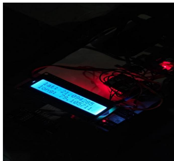
Fig. 10. GPS coordinates on 16*2 LCD screen
