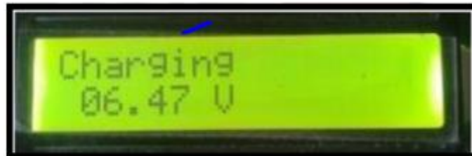
Figure 18. Voltage reading on LCD indicating flow of current.
