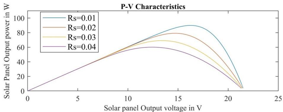
Figure 13 I-V Characteristics of Solar PV Panel at Various Series Resistance.
