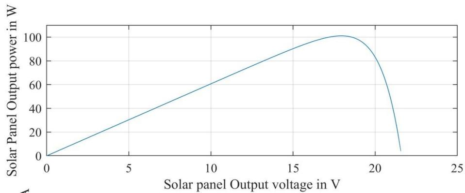
Figure 7 P-V Curve of Solar PV Panel at Standard Test Condition
