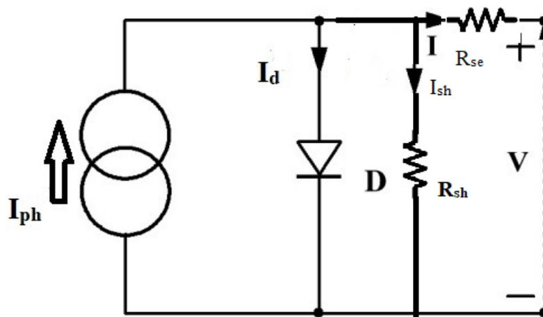
Figure 3 Equivalent Circuit of Five Parameters Single-Diode Solar PV Model
