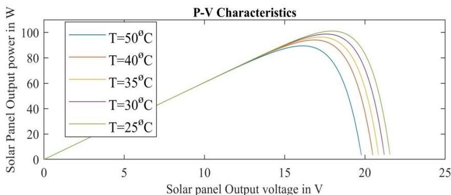
Figure 11 P-V Curves of Solar PV Panels at Various Temperatures
