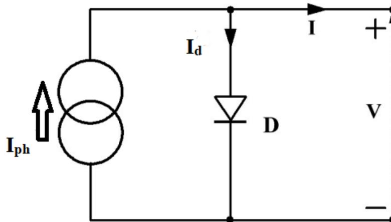
Figure 1 Model Equivalent Circuit for a Three-Parameter Single-Diode Solar PV
