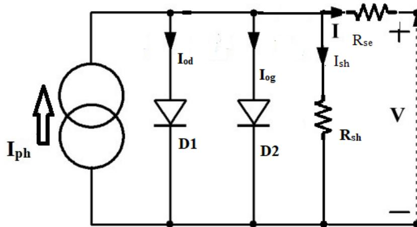
Figure 4 Equivalent Circuit of Seven Parameters Two-Diode Solar PV Cell
