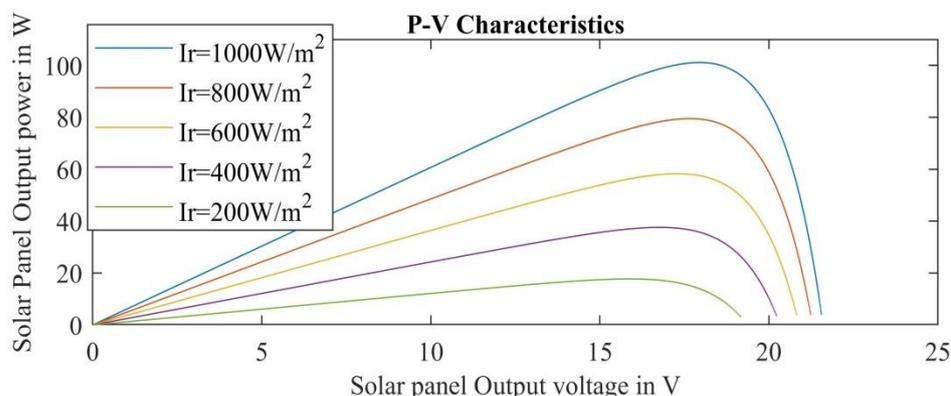
Figure 9 P-V Curves of Solar PV System under Various Solar Irradiation
