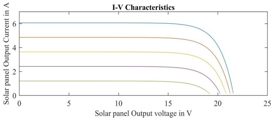
Figure 10 I-V Curves of Solar Module under Various Solar Irradiation
