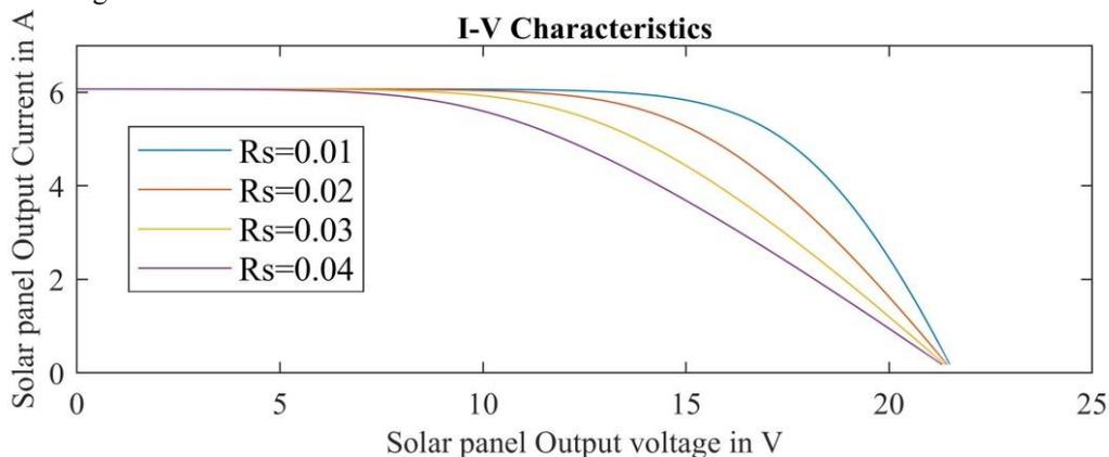
Figure 14 I-V Characteristics of Solar PV System at Various Series Resistance
