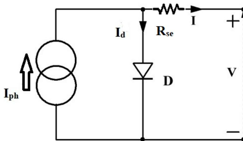
Figure 2 Model Equivalent Circuit for a Four-Parameter Single-Diode Solar PV Cell
