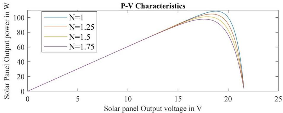
Figure 15 P-V Characteristics of Solar PV System at Various N
