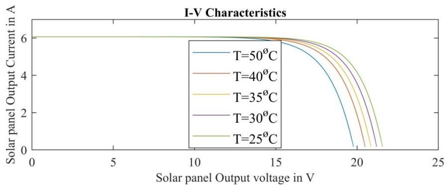
Figure 12 I-V Curves of Solar PV Panels at Various Temperatures
