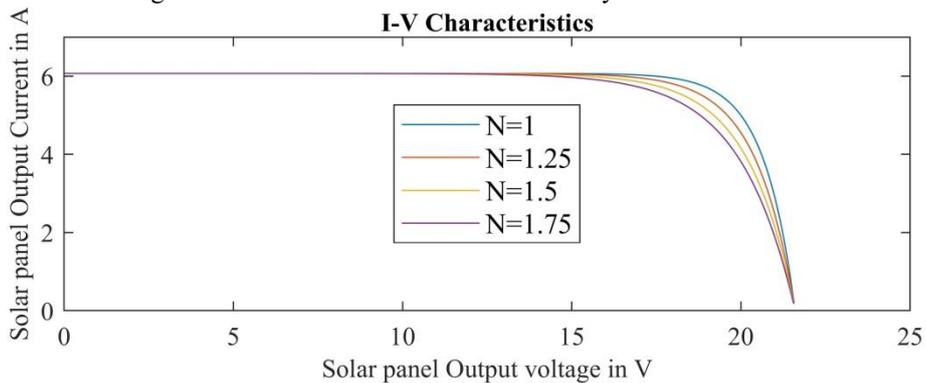
Figure 16 I-V Characteristics of Solar PV System at Various N
