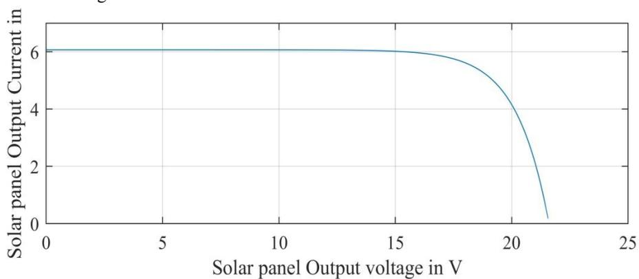
Figure 8 I-V Curve of Solar PV Panel at Standard Test Condition
