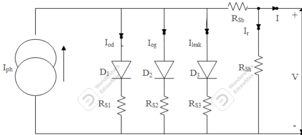
Figure 5 Equivalent Circuit of Three Diode Solar PV Model with Nine Parameters
