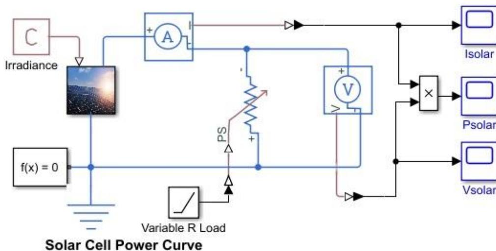
Figure 6 MATLAB Simulation Model of Solar PV System
