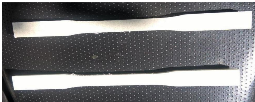
Fig.5 Specimen for Tensile and Compression test
