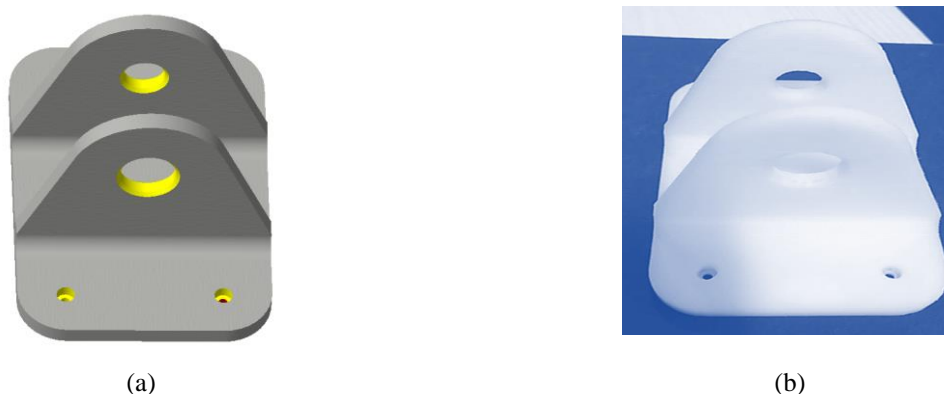
Figure 10: Photographs of the test artifact (a) CAD file with different Hole axis concerning the build direction, and (b) 3D-Printed Part to study the hole features.
