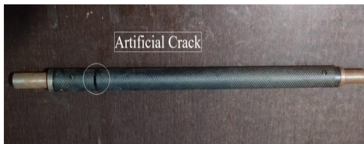
Fig.2 Artificial fracture on the Composite Drive Shaft
