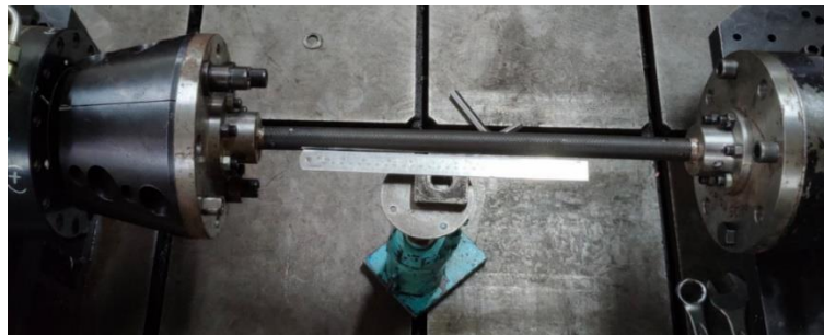
Fig.3 Torsional fatigue test set up of Composite Drive Shaft
