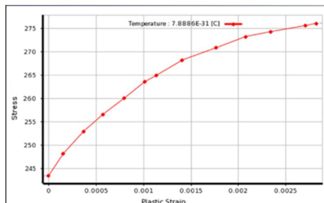
Figure 2 Multilinear Kinematic Hardening
