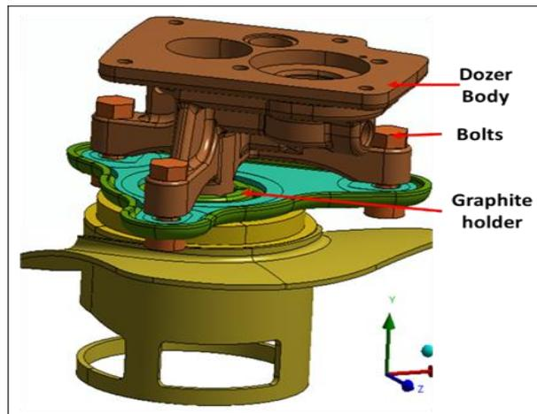
Figure 1 Geometric Details of DEF Dozing System
