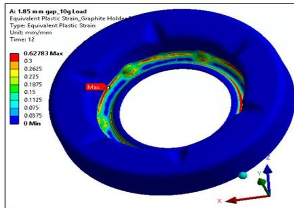
Figure 9 Plastic Strain at Graphite Holder
