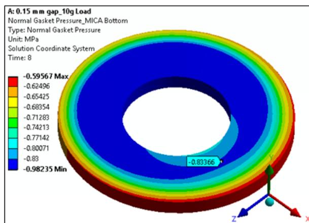
Figure 5 Minimum Gasket Pressure for MICA Gasket at Bottom
