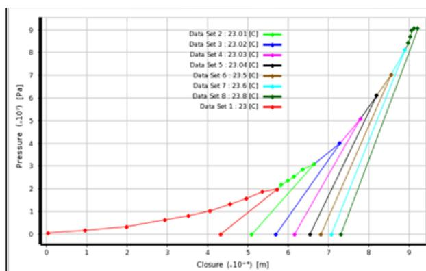
Figure 12 MICA Gasket-LD Curve
