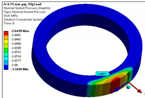
Figure 6 Minimum Gasket Pressure for Graphite gasket
