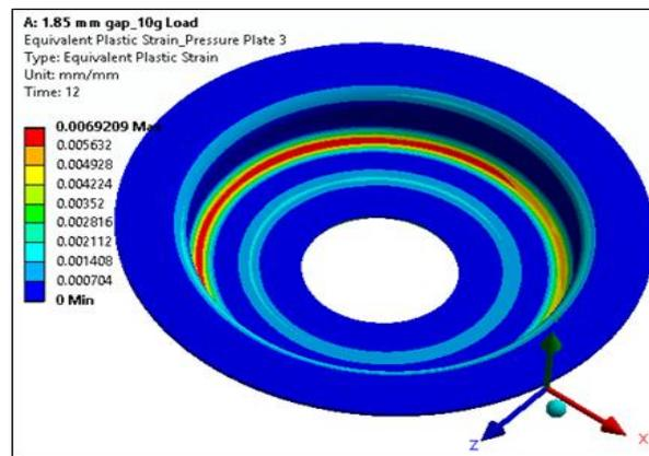
Figure 8 Plastic Strain at Retainer Plate
