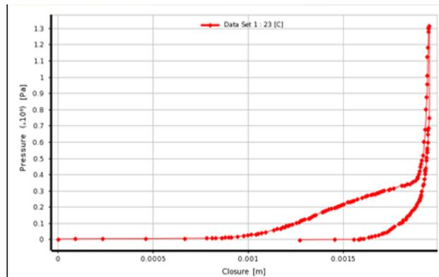
Figure 11 Graphite Gasket-LD Curve
