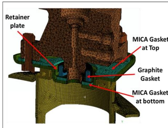
Figure 3 Mesh of the Assembly
