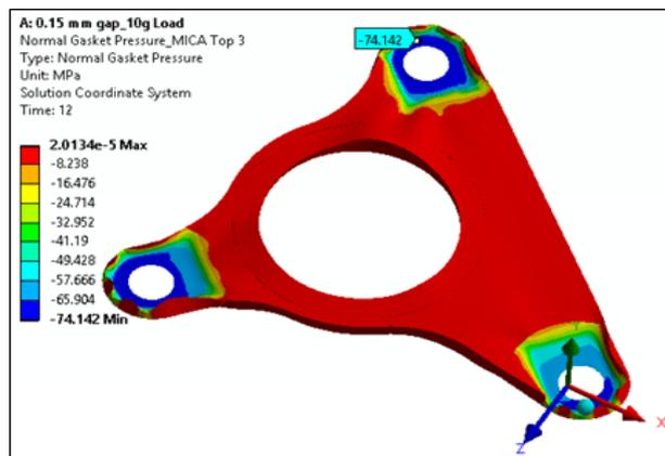
Figure 7 Maximum Gasket Pressure for MICA gasket at Top
