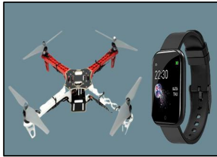
Figure 4. Hardware used in the trials includes a Mbientlab MetaWearR+ IMU bracelet on the right and a Bitcraze Crazyflie 2.0 quadrotor on the left.
