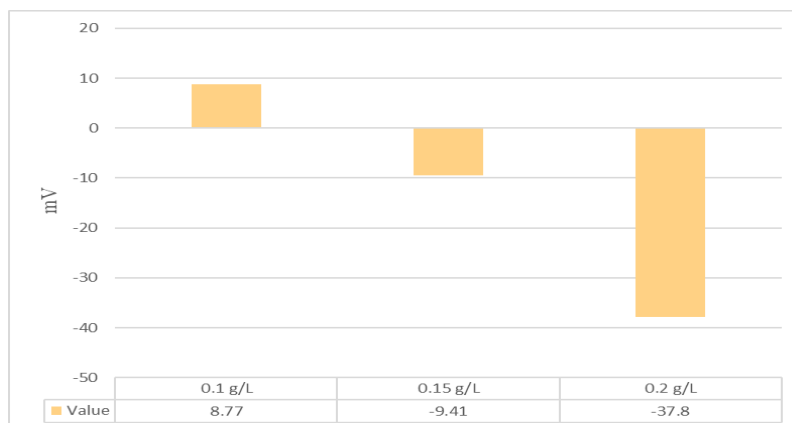
Figure 7. The result of Zeta Potential in graphene nano-lubricants
