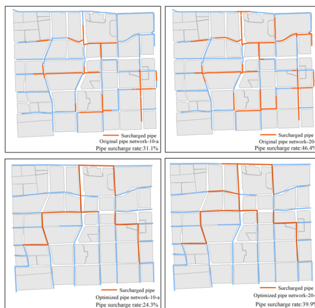
Fig. 9 Surcharged pipeline transmission. The percentage of a distance of a surcharged pipeline towards the overall length of the pipe is known as the pipeline surcharge rate.
