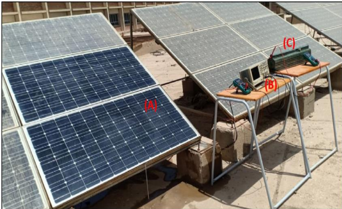
Fig. 4 Test Bed Setup for Solar PV Monitoring
