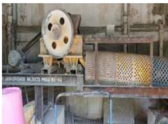
Figure 1: Equipment for Crushing & Processing Recycled Aggregates (With Screen Equipment)
